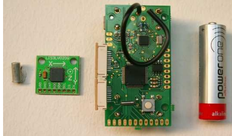
Figure 6.1: Movement sensors (left) and sensor node platform (right).
